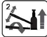
Pump to raise Undo valve to lower
