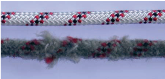
Fig. 2: Severe rope wear, wear with rope thickening
